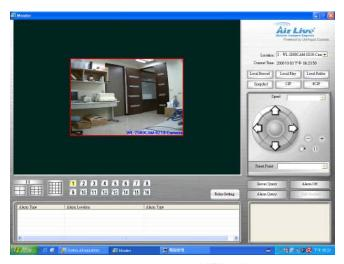
The CamPro Express allows you to monitor 32 channels via the computer and WEB UI. You can choose how you would like to view the camera, the Cam Pro Express supports 1/4/9/16/32 different view. You can also choose to view the different camera in single view or 1/4/9/16/32 view.
