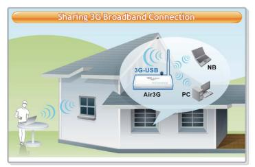
The Air3G comes with USB 2.0 port for sharing the Internet connection of 3G USB dongles. In addition, a WAN port is provided for sharing ADSL or Cable Modem connection. The remarkable WAN and 3G auto backup function will auto switch between WAN or 3G when one of the connections failed. This ensures uninterrupted Internet service for your home or office. Wireless Multi-mode functions can turn your Air3G instantly into AP, Wireless Client, Wireless Bridge, or Wireless Repeater.
