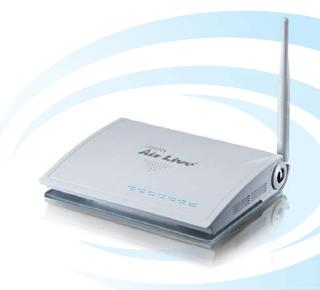
The Air3G is the latest AirLive AP router that follows the principles of maximization. It starts with earth shattering 1Watt output power\* that enables the AP to cover up to area of 1km in diameter. It is equipped with both USB and WAN port to share 3G, ADSL, and cable modem Internet connections. Hotspot authentication function is provided for those who want to resell the Internet bandwidth. The passive PoE port allows installation of the Air3G far away from power source.
